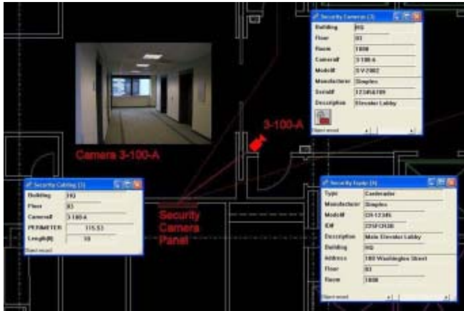
Figure 13 – Security Camera System (ArchiFM)
