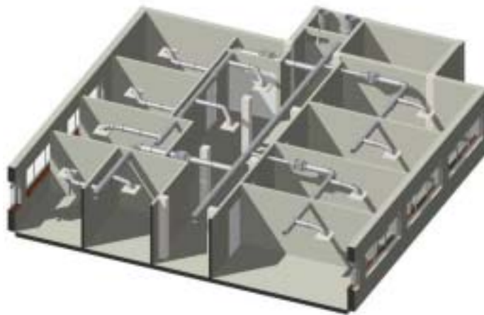
Figure 12 – 3D View of HVAC Ductwork (ArchiFM)
